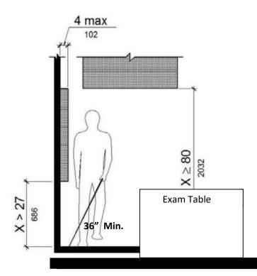
**Example:** A wall-mounted object protrudes into the 36" clear space as required by 11B-805.4.1.
